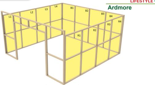
The above image shows the possible positions for PA doors. After selecting the desired position(s), use the dimensions specified in the following image to make PA door slope.
