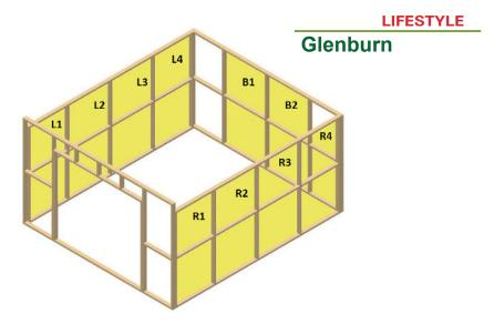
The above image shows the possible positions for PA doors. After selecting the desired position(s), use the dimensions specified in the following image to make PA door slope.
