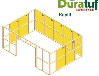
The above image shows the possible positions for PA doors. After selecting the desired position(s), use the dimensions specified in the following image to make PA door slope.
