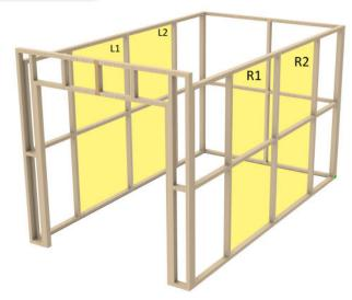
The above image shows the possible positions for PA doors. After selecting the desired position(s), use the dimensions specified in the following image to make PA door slope.
