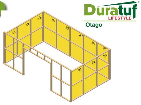
The above image shows the possible positions for PA doors. After selecting the desired position(s), use the dimensions specified in the following image to make PA door slope.
