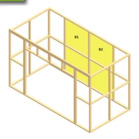
The above image shows the possible positions for PA doors. After selecting the desired position(s), use the dimensions specified in the following image to make PA door slope.
